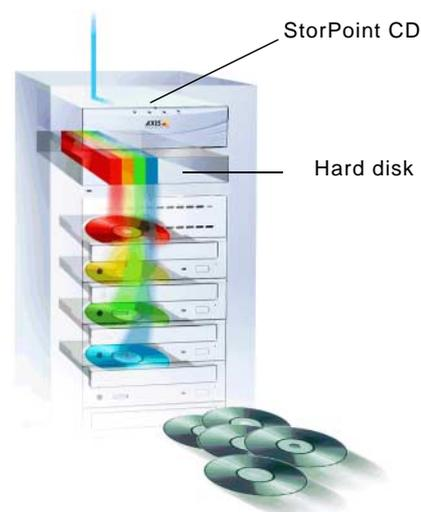
**Disc Changers** Because of the relatively long time needed to change discs in a changer, the data transfer rate may become unacceptably low when two users simultaneously attempt to read different discs. Hard disk caching will thus significantly increase the access speed if you are using changers.
