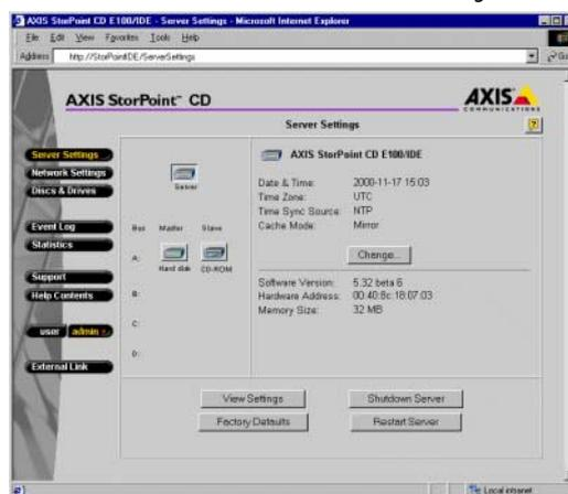
IDE Server - the icons displayed to the left represents all the units connected to the IDE bus listed as Master or Slave for each bus
